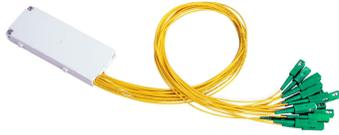
OCM6 Fiber Optic Splitter Module, Planar, three 1x8 Splitters, singlemode, LC/APC, symmetrical split ratio, butt style, 1.6 m pigtailed
