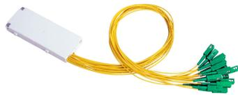
OCM6 Fiber Optic Splitter Module, Planar, one 1x64 Splitter, singlemode, SC/APC, symmetrical split ratio, butt style, 3 m pigtails
