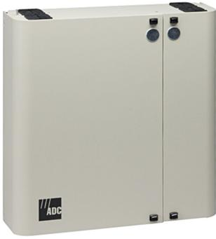
FL1000 Fiber Wall Box, 2-door, singlemode SC/UPC, 24-ports, with pigtails and splice tray, 1 cable clamp, 1 compression fitting, 1 grounding kit, 1 strength-member tie-off, 1 key lock
