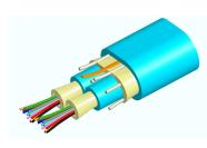
Fiber indoor cable, LazrSPEED®, Low Smoke Zero Halogen Riser MPO Trunk, 24 fiber with 12 fiber subunits, Gel-free, Multimode OM4, Feet jacket marking, Aqua jacket color, Dca flame rating
