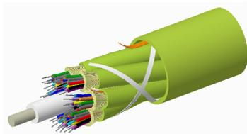
Fiber indoor cable, TeraSPEED® Plenum Distribution, 48 fiber multi-unit with 12 fiber subunits, Composite OM5 and G.652.D and G.657.A1, Gel-free, Feet jacket marking, Lime green jacket color
