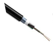
Fiber OSP cable, Multi-tube Cable with Corrugated Steel Armoring, OS2, 24-fiber with HDPE Jacket, Gel-filled, Singlemode G.652.D and G.657.A1, Meters jacket marking, Black jacket color
