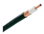
AVA6RK-50, HELIAX® Andrew Virtual Air<sup>™</sup> Coaxial Cable, corrugated copper, 1-1/4 in, black , fire retardant polyolefin jacket B2ca- s1b, d2,a1 (CPR testing is conducted annually please reference the website for latest classification)
