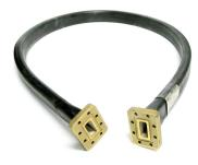
FlexTwist® Flexible Twist for WR137, 5.85–8.2 GHz, with interface types CPR137G and CPR137G, 900 mm
