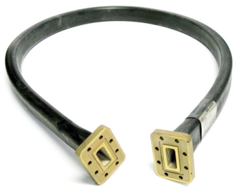
FlexTwist® Flexible Twist for WR137, 7.125–7.75 GHz, with interface types CPR137G and CPR137G, 600 mm
