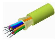
Fiber indoor cable, LazrSPEED® Low Smoke Zero Halogen Riser Distribution Cable, 4 fiber single-unit, Gel-free, Multimode OM5, Feet jacket marking, Lime green jacket color, B2ca flame rating
