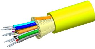
Fiber indoor cable, TeraSPEED® Low Smoke Zero Halogen Riser Distribution Cable, 4 fiber single-unit, Gel-free, Singlemode G.652.D and G.657.A1, Feet jacket marking, Yellow jacket color, B2ca flame rating
