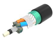
Fiber OSP cable, Outdoor Steel Armored, Gel-Free, Stranded Loose Tube Rollable Ribbon, 864 fiber, Singlemode G.652.D and G.657.A1, Feet jacket marking, Black jacket color, Build America Buy America (BABA)
