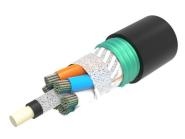
Fiber OSP cable, Outdoor Steel Armored, Gel-Free, Stranded Loose Tube Rollable Ribbon, 432 fiber, Singlemode G.652.D and G.657.A1, Feet jacket marking, Black jacket color, Build America Buy America (BABA)
