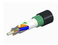
Fiber indoor/outdoor cable, TeraSPEED®, Single Jacket/Single Armor, Low Smoke Zero Halogen (LSZH), 144 fiber, Singlemode G.652.D and G. 657.A1, Gel Filled, Stranded Loose Tube, Black jacket color, Meters jacket marking, Cca flame rating
