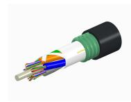
Fiber indoor/outdoor cable, TeraSPEED®, Single Jacket/Single Armor, Low Smoke Zero Halogen (LSZH), 48 fiber, Singlemode G.652.D and G. 657.A1, Gel Filled, Stranded Loose Tube, Black jacket color, Meters jacket marking, Cca flame rating
