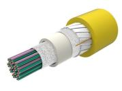
Fiber indoor/outdoor cable, All-Dielectric, LSZH, Riser-Rated, Gel-Free, Central Tube Rollable Ribbon, 144 fiber, Singlemode G.657.A2/B2, Feet jacket marking, Yellow jacket color, Cca flame rating
