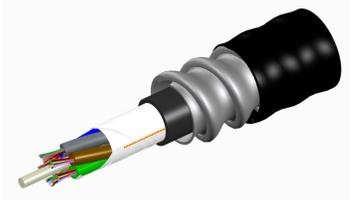
Fiber indoor/outdoor cable, LazrSPEED®, 12 fiber, Multimode OM5, Gel-Free, Stranded Loose Tube with Aluminum Interlocking Armor containing a Riser Rated Outer Jacket, Feet jacket marking, Black jacket color
