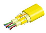
Fiber indoor cable, Low Smoke Zero Halogen Riser MPO Trunk, 24 fiber with 12 fiber subunits, Singlemode G.657.A2/B2, Gel-free, Feet jacket marking, Yellow jacket color, Dca Flame rating
