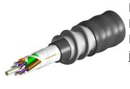
Fiber indoor/outdoor cable, TeraSPEED® Inner LSZH, Mini Stranded Loose Tube, Riser Rated, 72 fiber, Singlemode G.652.D and G.657.A1, Gel-Filled Subunits, Aluminum Interlocking Armor, Black jacket color, Feet jacket marking
