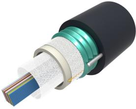
Fiber OSP cable, Steel Armored, Arid-Core, Dry Central Tube Ribbon, 192 fiber, Multimode OM3, bend insensitive, Feet jacket marking, Black jacket color
