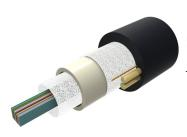
Fiber OSP Cable, Non-Armored, All-Dielectric, Arid-Core, 288 fiber, Dry Central Tube Ribbon, Singlemode G.652.D and G.657.Al, Gel-free, Feet jacket marking, Black jacket color
