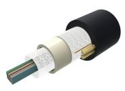
Fiber OSP Cable, Non-Armored, All-Dielectric, 144 fiber, Arid-Core, Dru Central Tube Ribbon, Singlemode G.652.D and G.657.A1, Gel-free, Feet jacket marking, Black jacket color
