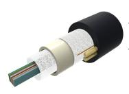
Fiber OSP Cable, Non-Armored, All-Dielectric, Arid-Core, Dry Central Tube Ribbon, 36 fibers, Singlemode G.652.D and G.657.Al, Gel-free, Feet jacket marking, Black jacket color
