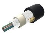
Fiber OSP Cable, Non-Armored, All-Dielectric, Arid-Core, Dry Central Tube Ribbon, 24 fibers, Singlemode G.652.D and G.657.Al, Gel-free, Feet jacket marking, Black jacket color
