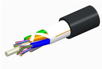
Fiber OSP cable, LightScope® ZWP Single Jacket All-Dielectric, 48 fiber, Gel-Filled, Stranded Loose Tube, Singlemode + Multimode OM3, Feet jacket marking, Black jacket color
