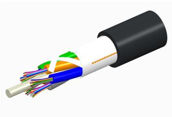
Fiber OSP cable, TeraSPEED® Single Jacket All-Dielectric, 96 fiber, Gel-Free, Outdoor Stranded Loose Tube w/HDPE Outer Jacket, Singlemode G.652.D and G.657.A1, Feet jacket marking, Black jacket color
