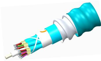
Fiber indoor cable, TeraSPEED® Plenum Distribution, interlocking aluminum armored with plenum jacket, Multimode/Singlemode, 48 fiber multi-unit with 12 fiber subunits, gel-free, Feet jacket marking, Aqua jacket color
