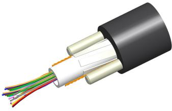
Fiber OSP cable, TeraSPEED® Single Jacket All-Dielectric, Gel-Filled, 2 fiber, Central Tube, Singlemode G.652.D and G.657.A1, Feet jacket marking, Black jacket color
