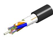
Fiber OSP cable, TeraSPEED® Light Duty, Single Jacket, All-Dielectric, 24 fiber, Gel-Free, Stranded Loose Tube, Singlemode G.652.D and G.657.Al, Feet jacket marking, Black jacket color
