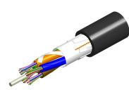
Fiber OSP cable, TeraSPEED® Light Duty, Single Jacket, All-Dielectric, 12 fiber, Gel-Free, Stranded Loose Tube, Singlemode G.652.D and G.657.A1, Feet jacket marking, Black jacket color
