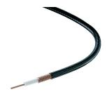
Heat Treated FSJ2RK-50, HELIAX® Superflexible Foam Coaxial Cable, corrugated copper, 3/8 in, black non-halogenated, fire retardant polyolefin jacket
