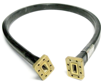
FlexTwist® Flexible Twist for WR62, 12.4–18.0 GHz, with interface types UG-419/U and PBR140, 600 mm
