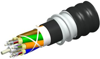
Fiber indoor/outdoor cable, LazrSPEED® Riser/LSZH rated, Distribution, interlocking aluminum armored, 6 fiber single-unit, Multimode OM3, Gel-free, Feet jacket marking, Black jacket color
