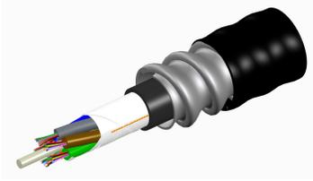
Fiber indoor/outdoor cable, LazrSPEED®, Gel-Free, 12 fiber, Stranded Loose Tube with Aluminum Interlocking Armor containing a Riser Rated Outer Jacket, Multimode OM3, Feet jacket marking, Black jacket color
