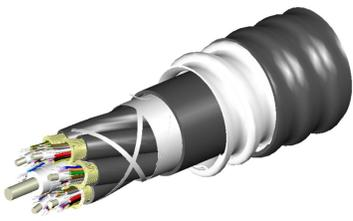
Fiber indoor/outdoor cable, TeraSPEED® LSZH Riser Distribution, interlocking aluminum armored, 36 fiber multi-unit with 12 fiber subunits, Singlemode G.652.D and G.657.A1, Gel-free, Feet jacket marking, Black jacket color
