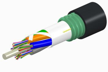
Fiber indoor/outdoor cable, TeraSPEED®, Single Jacket/Single Armor, Low Smoke Zero Halogen (LSZH), 24 fiber, Singlemode G.652.D and G.657.A1, Gel-Free, Stranded Loose Tube, Black jacket color, Feet jacket marking, Cca flame rating
