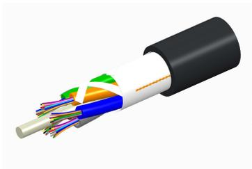
Fiber indoor/outdoor cable, TeraSPEED®, Single Jacket All-Dielectric, Low Smoke Zero Halogen (LSZH), 6 fiber, Singlemode G.652.D and G.657.A1, Gel-Free, Stranded Loose Tube, Black jacket color, Feet cable marking, Eca flame rating
