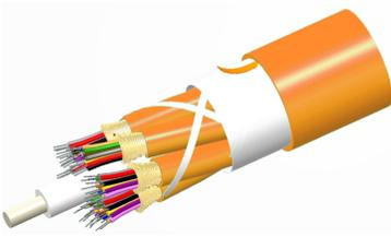
Fiber indoor cable, TeraSPEED® Riser Distribution, 36 fiber multi-unit with 12 fiber subunits, Singlemode G.652.D and G.657.A1, Gel-free, Feet jacket marking, Orange jacket color
