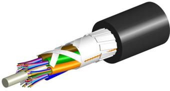
Fiber indoor/outdoor cable, LazrSPEED®, Mini Single Jacket, All-Dielectric, Riser/LSZH rated, 144 fiber, Gel-Filled, Stranded Loose Tube, Multimode OM3, Feet jacket marking, Black jacket color, Eca flame rating
