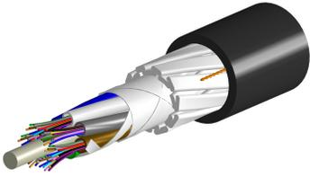
Fiber indoor/outdoor cable, LazrSPEED® High Tensile Strength Riser /LSZH Rated Mini All-Dielectric Single Jacket, Gel-Filled, 48 fiber, Stranded Loose Tube, Multimode OM3, Feet jacket marking, Dca flame rating. Provides Rodent Resistance
