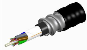
Fiber indoor/outdoor cable, TeraSPEED® Riser Rated, 288 fiber, Singlemode G.652.D and G.657.A1, Gel-Free, Stranded Loose Tube with Aluminum Interlocking Armor containing a Riser Rated Outer Jacket, Black jacket color, Feet cable marking
