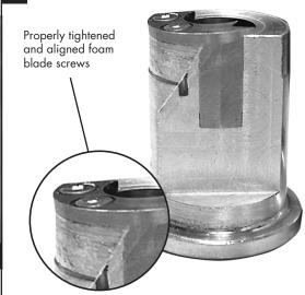
Ensure that the screws on the Foam blade are aligned and tightened down properly. Make sure the screws don't appear to be sitting up.
