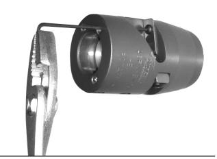
Unscrew the flat blade using a plier for leverage and replace it with the new flat blade. Repeat same to replace jacket blade.
