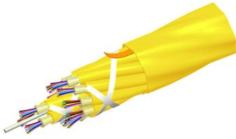
Fiber indoor cable, Low Smoke Zero Halogen Riser MPO Trunk, 96 fiber with 2.0 mm Subunits, Singlemode G.657.A2, Feet jacket marking, Yellow jacket color, B2ca flame rating
