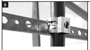
Insert front latches into the 3/4" hole and release.
