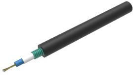
Fiber OSP cable, LightScope® ZWP Single Jacket/Single Armor, Gel-Filled, 4 fibers, Central Tube Cable, Singlemode G.652.D and G.657.A1, Custom jacket marking, Black jacket color
