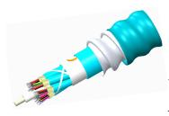
Fiber indoor cable, TeraSPEED® Low Smoke Zero Halogen Riser Distribution, interlocking aluminum armored, Multimode/Singlemode, 36 fiber multi-unit with 12 fiber subunits, Gel-free, Feet jacket marking, Aqua jacket color
