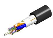
Fiber indoor/outdoor cable, LazrSPEED®, Light Duty, Single Jacket, Riser Rated, Multimode OM4, Gel-Free, All-Dielectric Outdoor Stranded Loose Tube, 36 fiber, Feet jacket marking, Black jacket color
