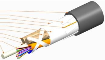
Plenum-Rated Outer Jacket Strength Elements Binder Water Swellable Tape Ripcord (1) Binder 2.5 mm Gel-Free Buffer Tubes 250 micron Fibers
